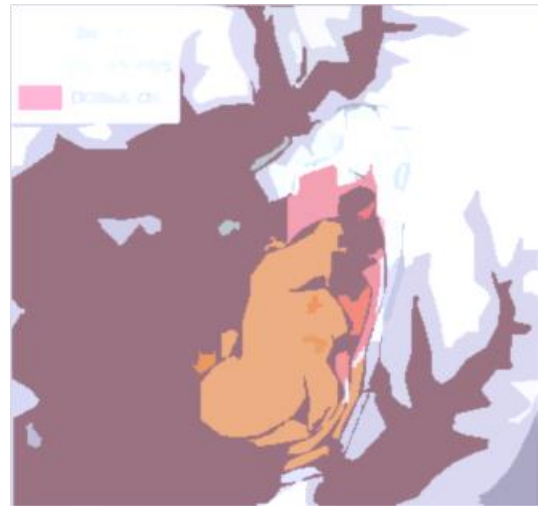
Fig- 4: Map overlap including the final fire predictions applying both DDDAS schemes and the real fire spread
