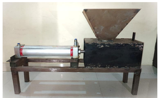
Fig 2. Working Model of Scrap Compressor
