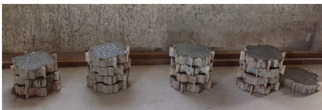
Fig-1: Casted Paver Blocks
