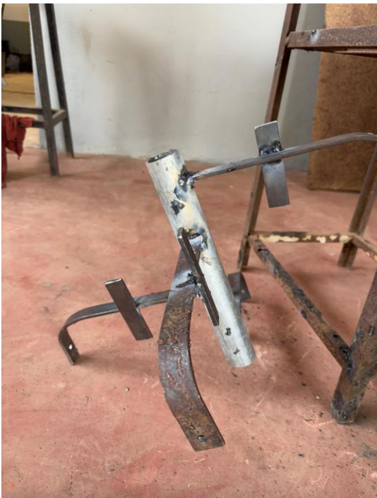
Fig -2: Mixing Blade Of Concrete Mixture
