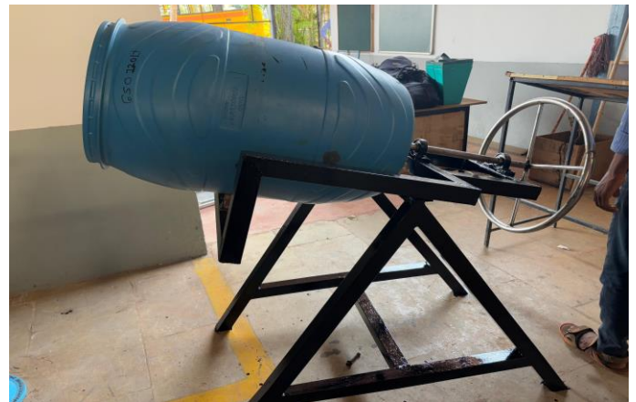
Fig-3: Mixing Drum Mounted on Framed Structure
