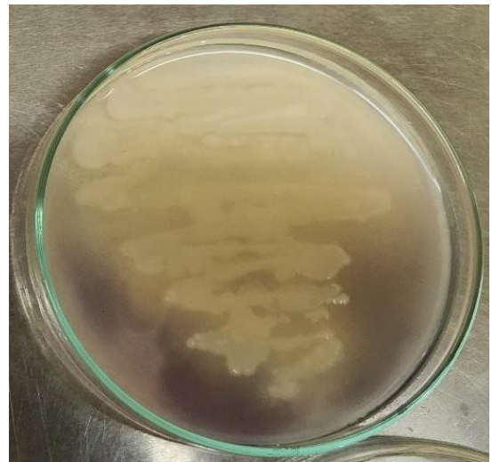
Fig. 9 A clear zone around the bacterial growth was observed, indicating starch degradation, while the remaining starch reacted with iodine to produce a dark brown coloration.
