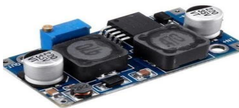
Fig No. 6: DC - DC Boost Convertor.
