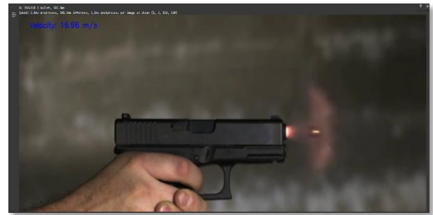
Fig -8: High velocity projectile detection and velocity estimation using video analysis YOLO model
