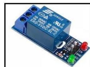
Fig-3: Relay Module
