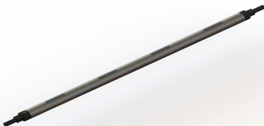
Fig - 4.1: Pneumatic Expansion Shaft 3d Assembly
