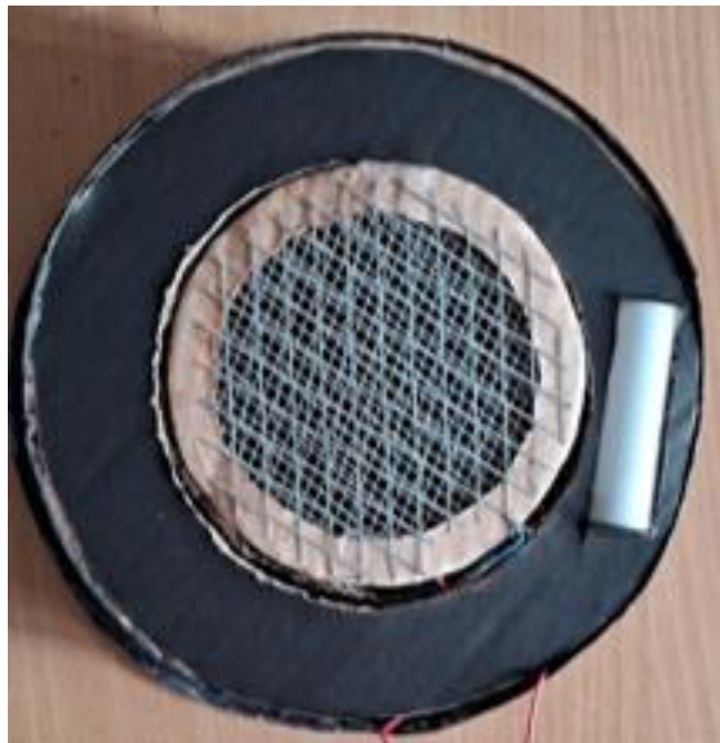
Fig -1: Top view of the prototype showing the mesh grid and UV LED arrangement.
