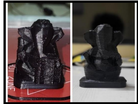
Figure 9: Better surface finish due to presence of supports on Lord Ganesha 3D model
