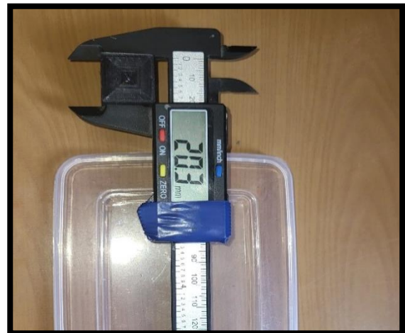
Figure 5: Calibration cube measured with digital vernier caliper
