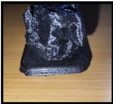
Figure 8: Visible layer lines on incomplete Lord Ganesha 3D model due to absence of supports
