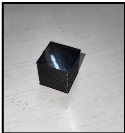
Figure 4: 20 × 20 mm Calibration Cube
