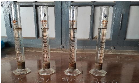
Fig 3.1 : Differential Free Swell Test
