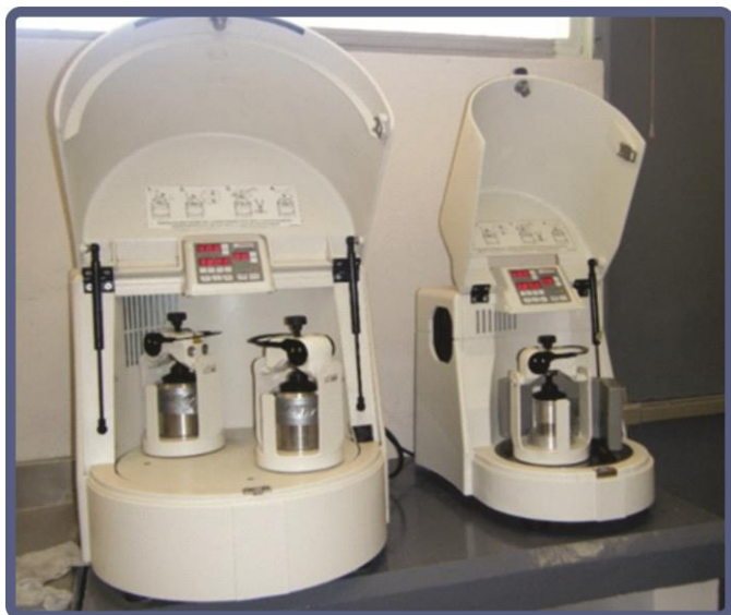
Figure 1: Fritsch Pulverisette 5 and 6 high-energy planetary mills, each equipped with a 65 ml bowl.
