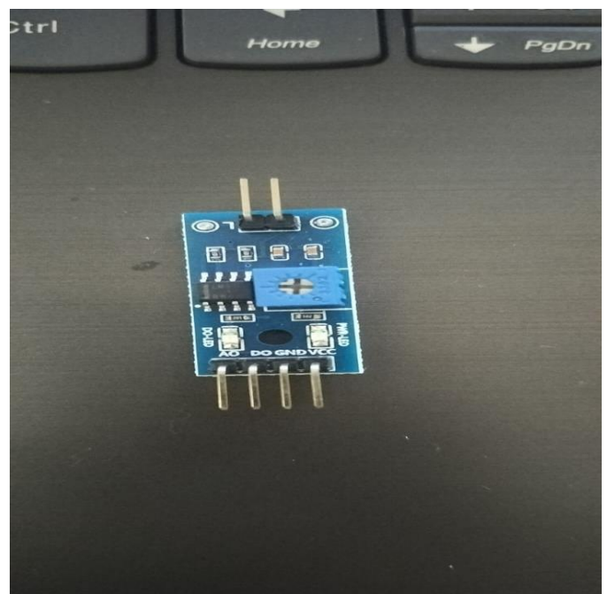
figure -1: Rain Sensor module
