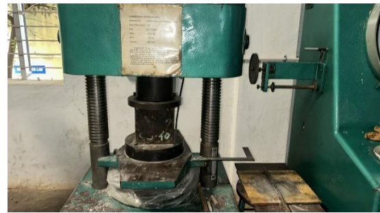
Figure 3 Compressive Strength Testing
