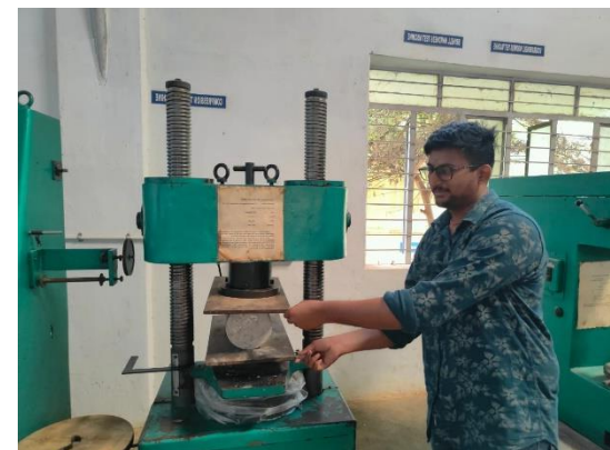
Figure 4 Split Tensile Test
