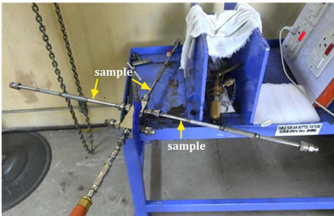
Fig-12: Pneumatic Leak Testing in progress
