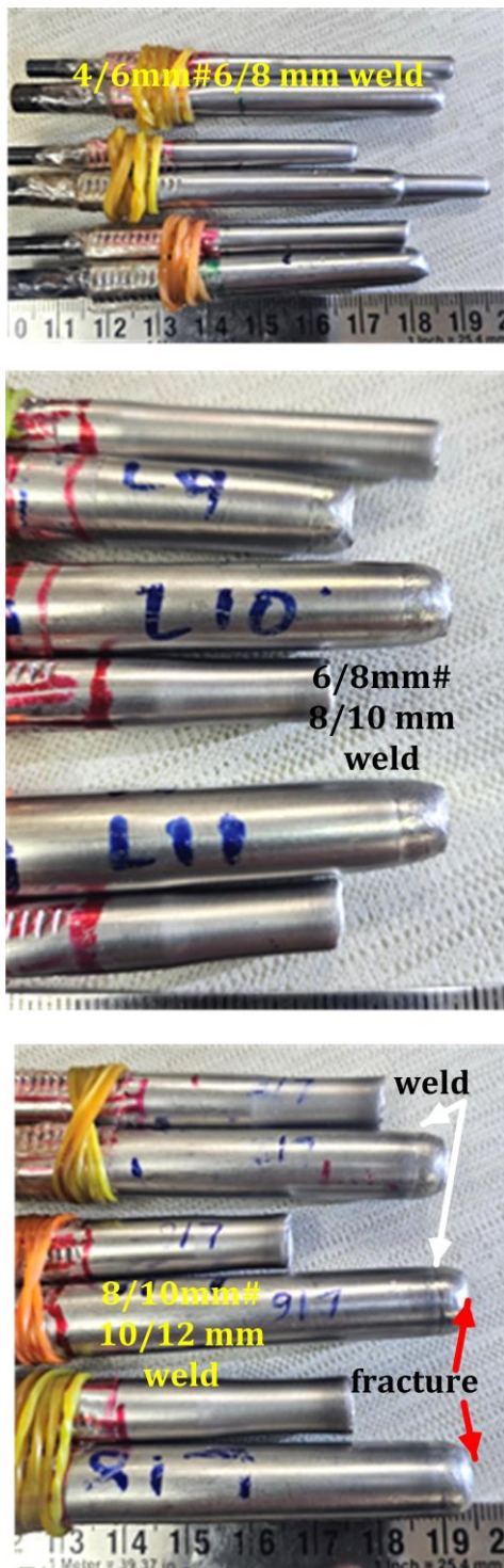
Fig-15: Failure location in tensile tested weld joints
