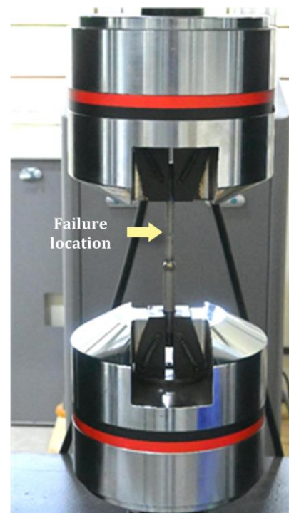
Fig-14: Fracture location of 9/12mm#13/16mm joint during tensile testing
