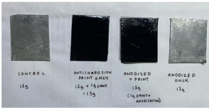
Fig -1: Photographs of test specimens before immersion testing: (a) untreated control (b) anodized only (c) painted only and (d) anodized then painted specimens.
