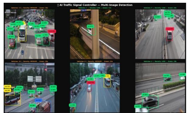
Fig.2: Multi-image vehicle detection and traffic density analysis
