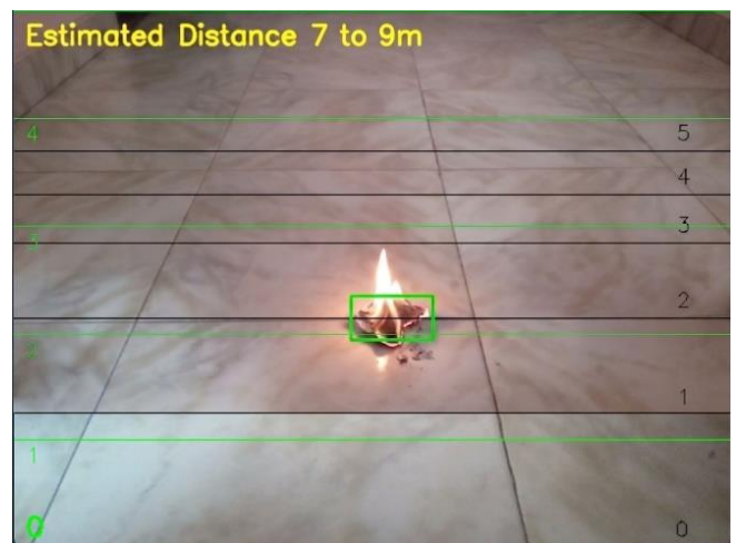
Fig -5. Sample system output showing detected object and estimated distance range overlaid on the camera frame.
