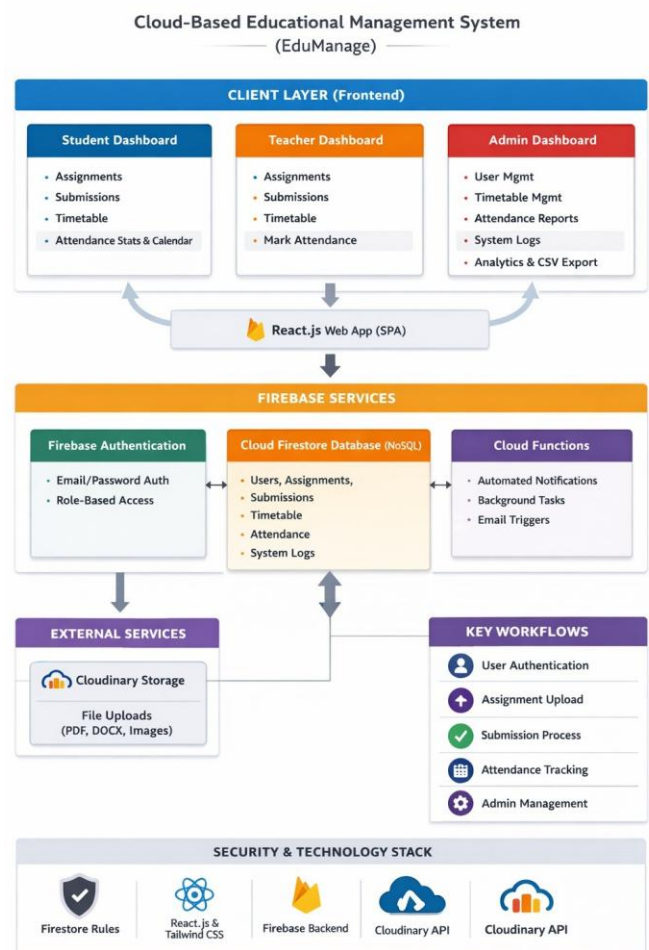
Fig -1: System Architecture
