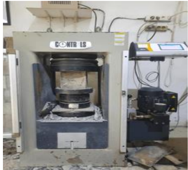
Fig 1 Compressive Strength testing
