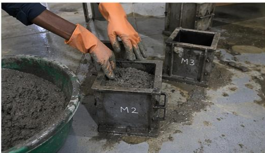
Fig. 5. Cube Casting Process
