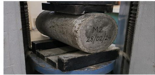
Fig. 7: Compression Testing in UTM
