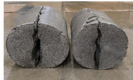
Fig. 8. Failure Pattern of Specimens
