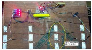
Fig.5. Experimental set up and testing under line to line to line fault condition
