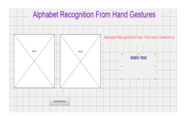
In our project we have created GUI as shown in above fig. We have taken two axes control to show captured image and the edge detected image of the input image. We have created the push button to capture the image through webcam and also added the static text box to show the corresponding text of the gesture.
