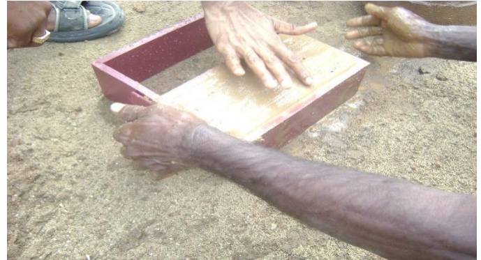
Fig.2.2 Finish of Moulding
