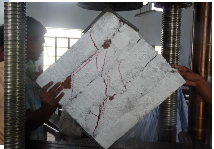
FIG.3.3.REINFORCED SPECIMEN - DUCTILE FAILURE
