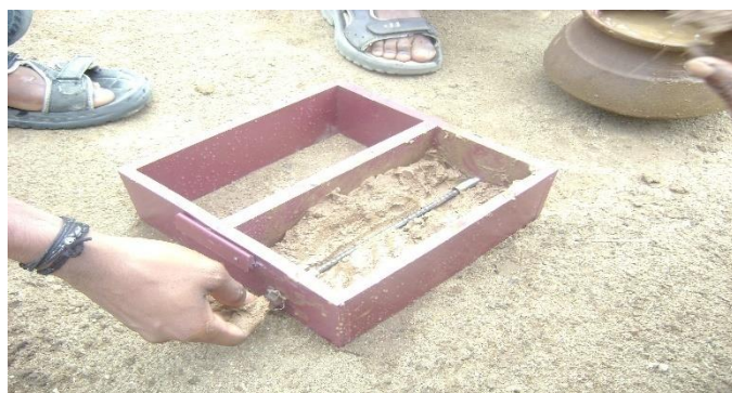
Fig.2.1 Insertion of 6 mm dia rod while moulding of bricks
