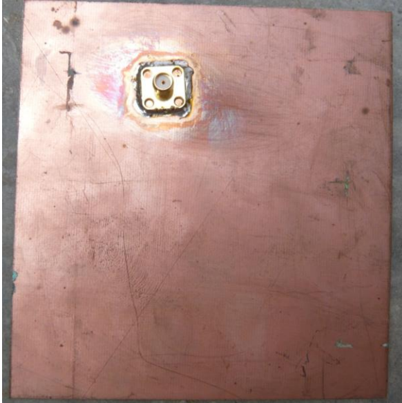
Figure 12: Rectangular microstrip patch antenna resonating at 1.09 GHz.
