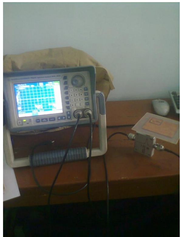
Figure 15: Connection of CircleHead MSA through SWR Bridge to Spectrum analyzer.
