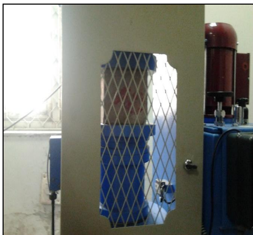
Fig. 4: Compressive Strength Testing under 200T CTM
