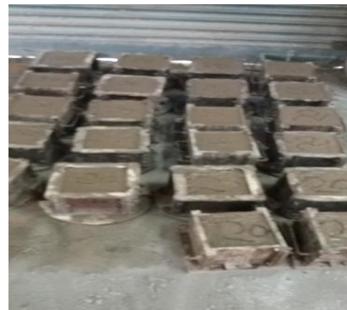
Fig. 2: Casting of Cubes
