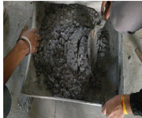
Fig. 1: Mixing of multiblend Concrete
