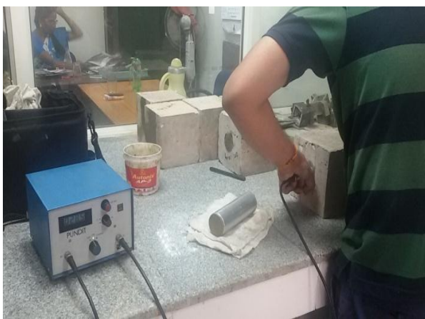
Fig. 3: Non Destructive Testing using Ultrasonic Pulse Velocity Method
