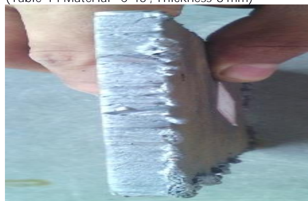
(Fig.18 Gas cutting by LPG) (Table-15 Material –C-45, Thickness-8 mm)
