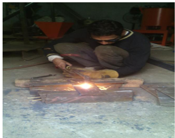
(Fig.5 working of gas cutting on C-45 material)
