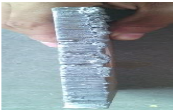
(Fig.20 Gas cutting by LPG) (Table-17 Material -C-45, Thickness-10 mm)
