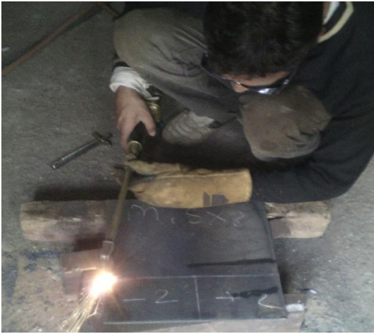
(Fig.6 working of gas cutting on M.S. material)
