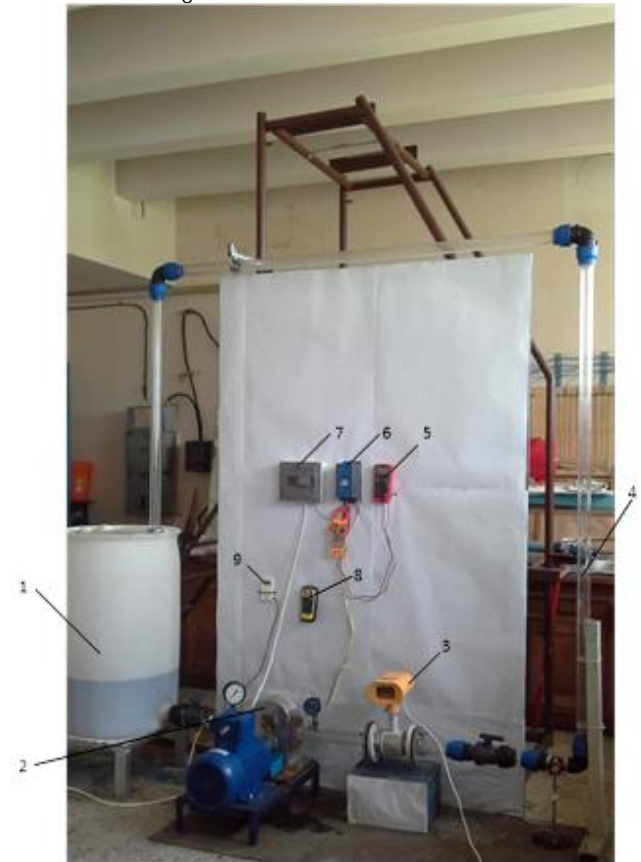
Fig -3: General overview of the installation 1- tank with fluid; 2- rotating volumetric pump; 3- electromagnetic flow meter; 4- transparent plexiglass pipe; 5- multimeter; 6- frequency converter; 7- fuse box; 8- differential manometer; 9- digital thermometer
