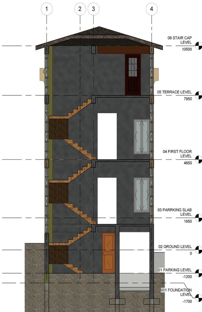
Fig -11: Section Cutting Staircase Room-1
