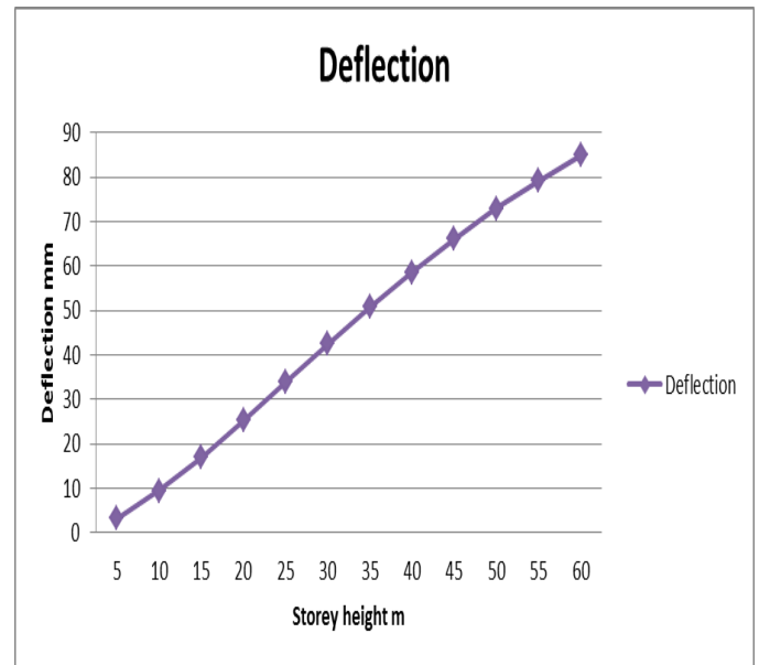
Fig.6.2: Graph showing Deflection at various floors.
