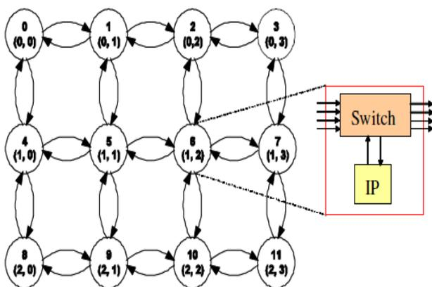
It is one of the easiest topologies to implement on a silicon die, because of its flat configuration. Mesh size given as  $R \times C$  means the number of node rows is  $R$  and the number of node columns is  $C$ . Cube and hypercube are also regular topologies similar to mesh.
