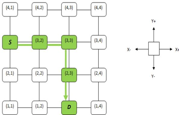
Allows path in XY routing algorithms.
