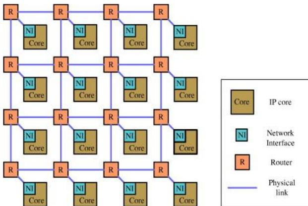
Network-On-Chip (NoC) consists of IP core, Network interfaces, routers, links. In NoC each core is connected to a switch by a network interface. The function of a network interface that define how data packets are formatted for transmission and routing. Routers direct data over several links (hops). Links connect switches with network interfaces or with other switches. NoC architecture consists of various topology as: Mesh, Ring, Torus, Star etc.
