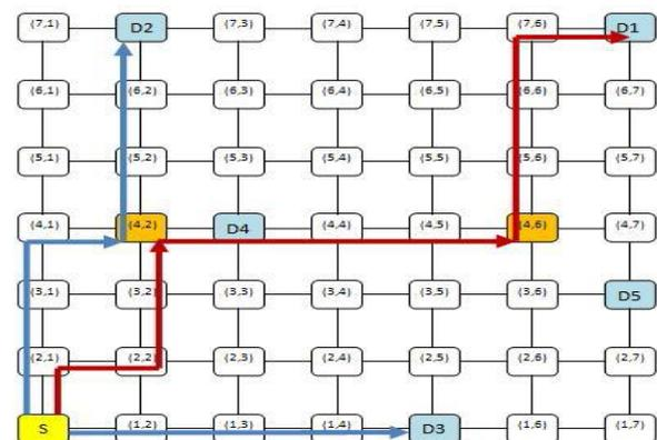
The node that is presented using (x,y) is located at xth row and yth column. Distance between nodes that is located at position (x1, y1) and (x2, y2) is calculated using the formula:
