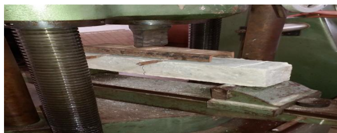
Fig-4.2: Split tensile test
