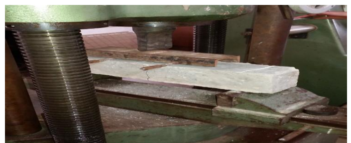
Fig-4.3: Flexural test
