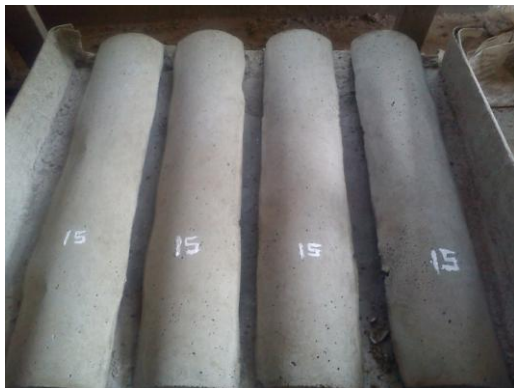
Fig 2.1(b): Segmental concrete pieces which are to be attached to square columns
