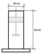
Figure 1: Bench Scale Model Setup
