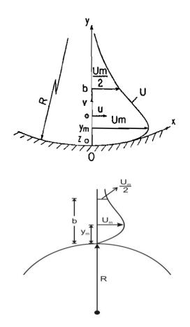
Fig. 2 Definition sketch of curvature parameter b/R
