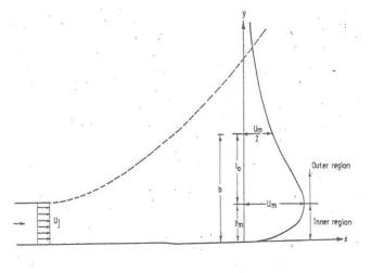
Fig.1 Definition sketch of a wall jet
