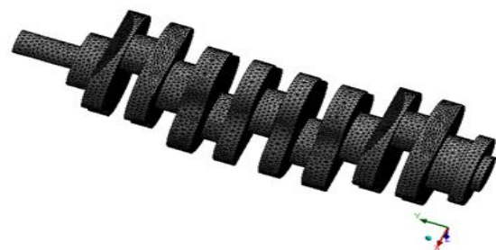
Figure-2.5: Meshed Model of forged steel crankshaft
