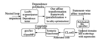
Fig -4: Source to source-to-source transformation system [8]
