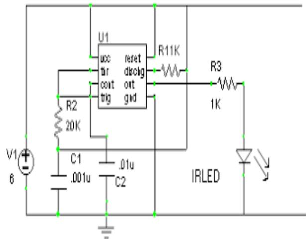
The power supply for transmitter is derived from the receiver is powered by regulated 6V dc.For this purpose you can use a 6V battery.
