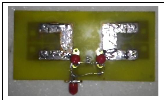
FIG. 16 PHOTOGRAPH OF GROUND PLANE OF ARRAY
