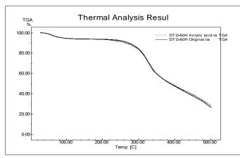
Figure 7 Thermogram analysis of Original (control) silk and AA-grafted-silk
