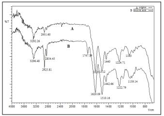
Figure 5 FTIR spectra of Original silk and Acrylic acid grafted silk
