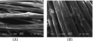
Figure 6 Scanning electron micrographs of ungrafted silk (A) and AA-grafted-silk (B)
