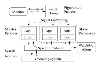
FIG.2-overview of the PLR system architecture with Three redundant processes.
