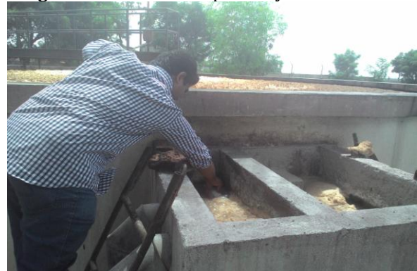
Fig -2: Wastewater sample collection from clarifier
