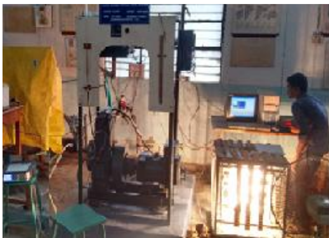
Fig -4: Computerized, four stroke single cylinder CI engine with Electrical loading
