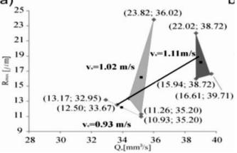
Chart 1(a) - average roughness value  $R_a$  vs. material removal rate Q in D181 tool.
