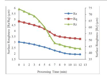
Figure 2. Representation of R<sub>a</sub> vs. processing time
