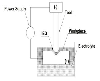
Figure.1. Schematic diagram of ECM process
