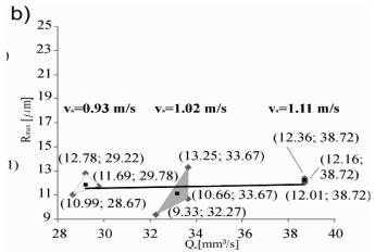
Chart 1(b) - average roughness value  $R_a$  vs. material removal rate Q in D151 tool.
