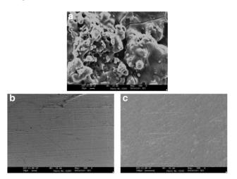
Figure 3- Representation of the typical SEM analysis (a – before machining, b – after micro grinding, c – after ECH).
