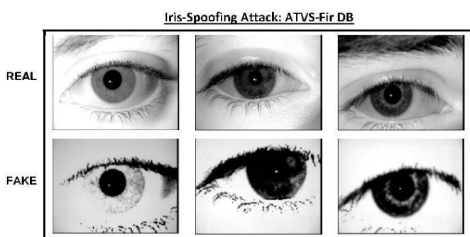
Fig-4: Typical real iris images (top row) and their corresponding fake samples (bottom row) that may be found in the ATVS-FIr DB used in the iris-spoofing experiments. The database is available at http://atvs.ii.uam.es/ .
