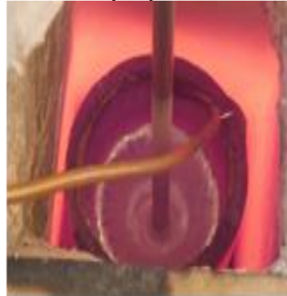
Fig-2: Stir Casting by Vortex Method
