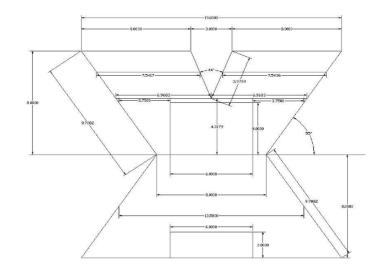
**Fig-4:** Design of the Main Part of Rocket Stove (measurement in inches)
