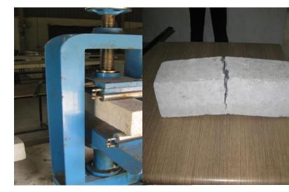
Fig 3: Testing of Prism
