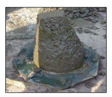
Fig 2: Slump test
