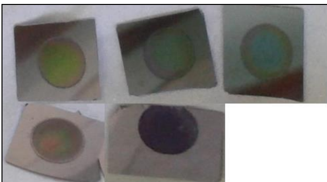
Fig -2: Electrochemically fabricated porous silicon samples with various etching time
